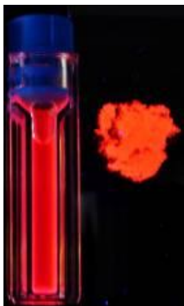
Fig. 1 Red fluorescence of BSA-Gold nanoclusters in aqueous solution and powder form under UV light.
